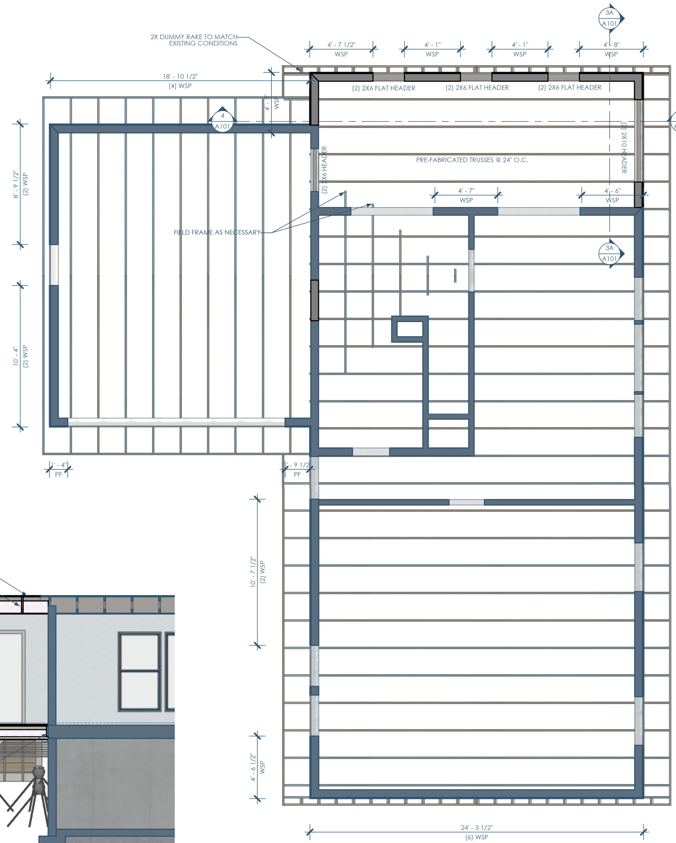
2A/A101 RCP - ROOF FRAMING 1/4"=1'-0"
