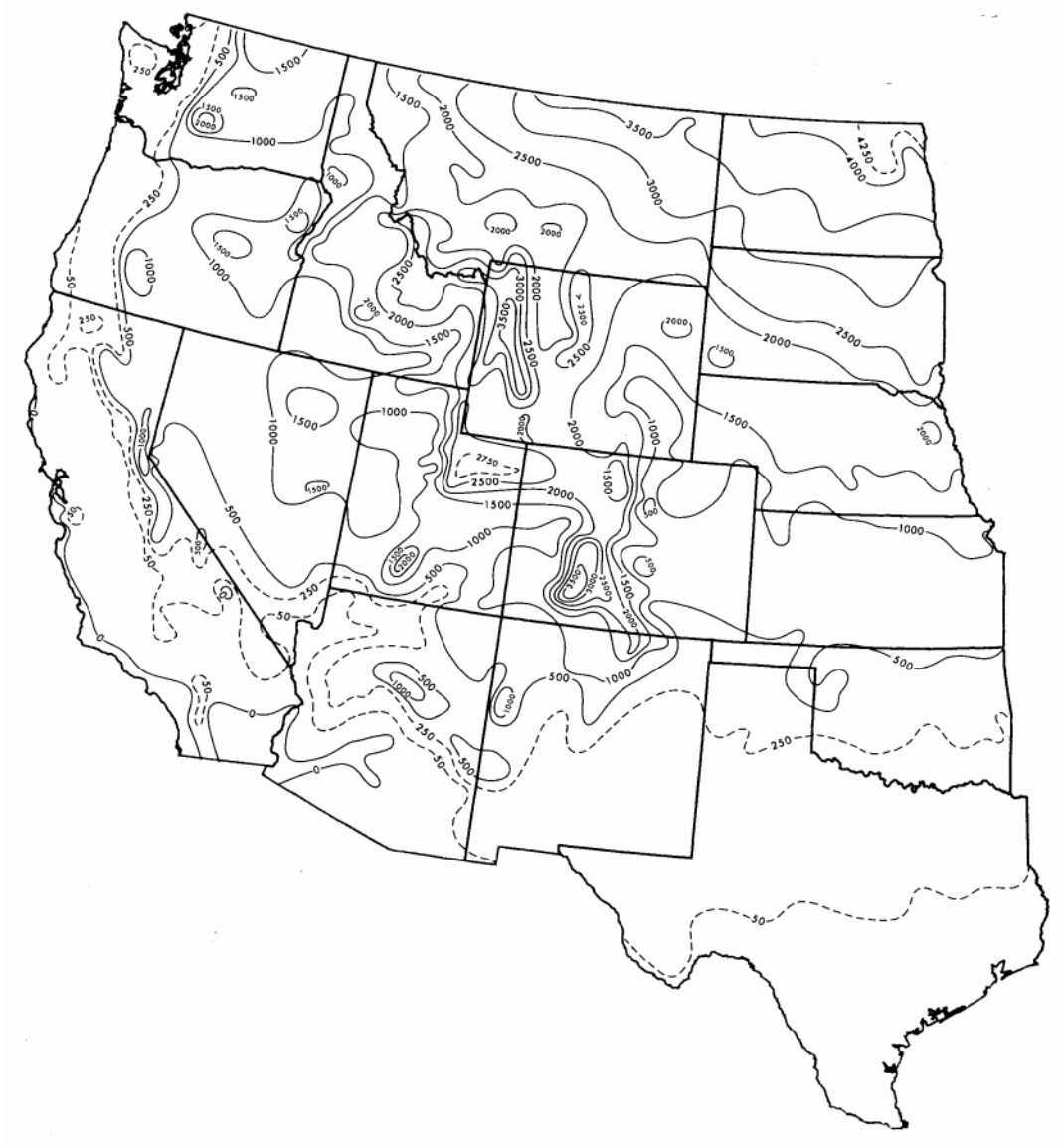
FIGURE A1. United States Design Air-Freezing Index (°F-Days) Contour Map (an Estimate of the 100-Year Mean Return Period), F_{100}
